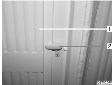
Fig. 108 Lock, toilet compartment panelling
