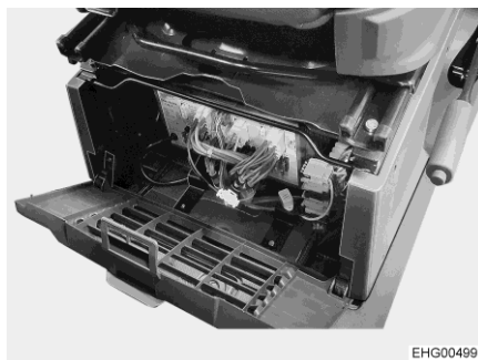
Fig. 94 Position of the transformer/rectifier
